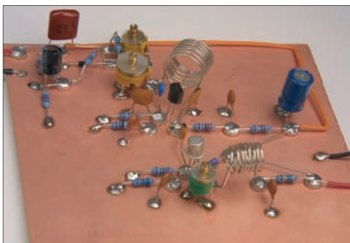
● The simple 70MHz transmitter project...which will provide 'first time' v.h.f. constructors with some interesting practice!
